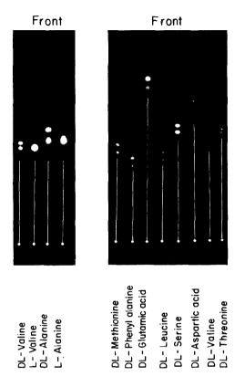
Figure 1. Dansyl amino acids resolved to enantiomers by treated reversed-phase TLC plates, spotted with 1 µ1 of ~5 10<sup>-4</sup>M solution. Plate length is 20 cm. Photographed under U.V. illumination.
